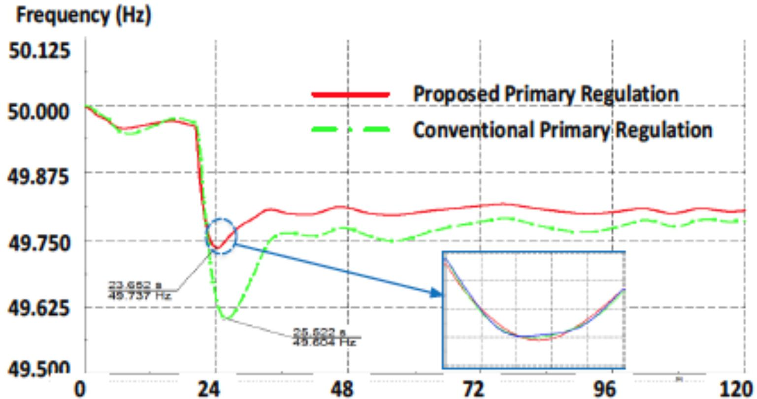
Fig. 9. Simulation result of the proposed VESS based primary frequency regulation
